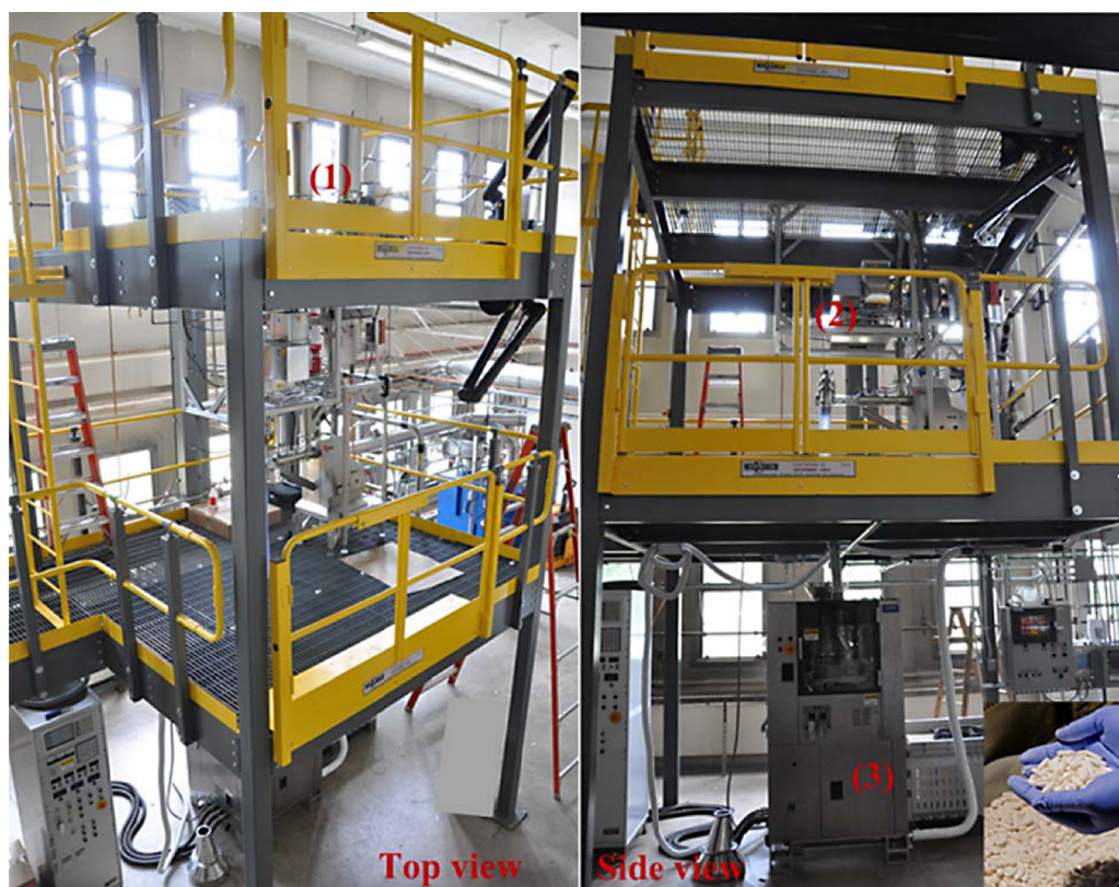
Fig. A1. Continuous direct compaction tablet manufacturing pilot plant (adapted from Singh et al., 2012b).
