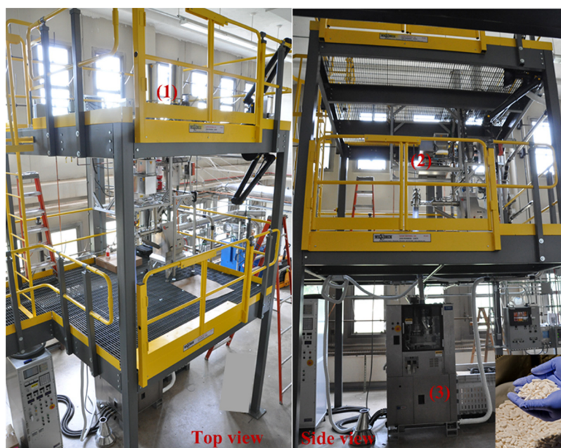
Fig. 3. Direct compaction tablet manufacturing pilot plant (adapted from Singh et al., 2012b) (whole plant is not shown): (a) feeders, (b) blender, (c) tablet press.
